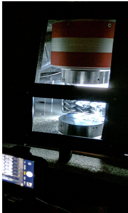
Left: Contact-free metrology using polarized light and mechanical testing of metamaterials with the Instron.
