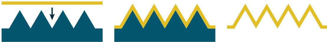
**Figure A1:** In vacuum thermoforming a heated polymer sheet is placed on a mold which then applies a vacuum, pulling the sheet into full contact with the mold surface. After a predetermined amount of time the mold is released and the finished part is ready for trimming.
