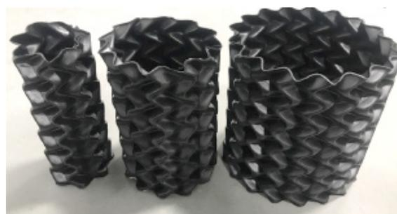
**Orientation Y Cylinders:** Y-axis parallel to the axis of the cylinder and thinner valley side of the thermoformed sheet on the exterior.
