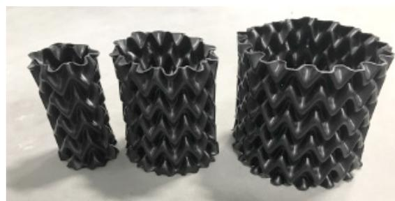
**Orientation X Cylinders:** X-axis parallel to the axis of the cylinder and thicker mountain side of the thermoformed sheet on the exterior.
