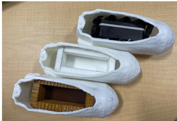
**Figure 23:** Given the fractured and nascent market for UAV medical delivery, we designed a generic UAV shell to act as a surrogate for existing systems. A render of the shell is shown in the top image, and 3 cast replicates are shown in the photograph below. These three replicates are housing HDPE MetaCORE [MO] (black material), foam (white material), and honeycomb (amber material). The 3-axis accelerometer is in the UAV loaded with MetaCORE and ready to be sealed for drop testing.
