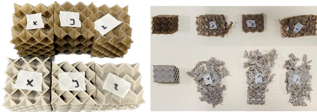
**Figure 16:** Photographs of 3D printed MetaCORE [MO] made from PEEK. The darker amber are as-printed, whereas the lighter beige is the appearance after annealing. Notice the difference in number of discrete pieces in the samples that were crushed to failure. While annealing does not measurably affect the modulus or strength, the annealing causes the post-yield behavior to go from ductile-like to brittle-like.
